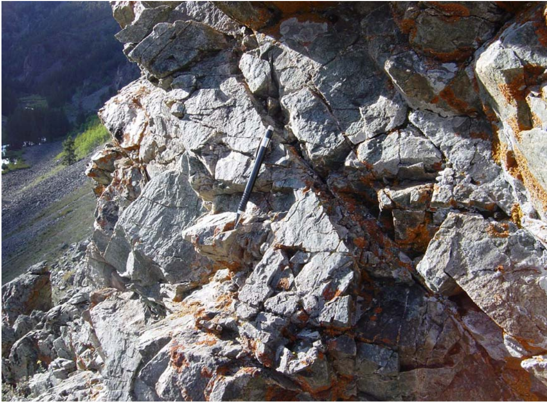
Photo 2.5 Closely spaced fractures; Outcrop Area 1.
