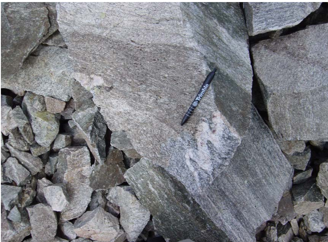
Photo 2.4 Foliation and minor fold structures in gneissic rock
