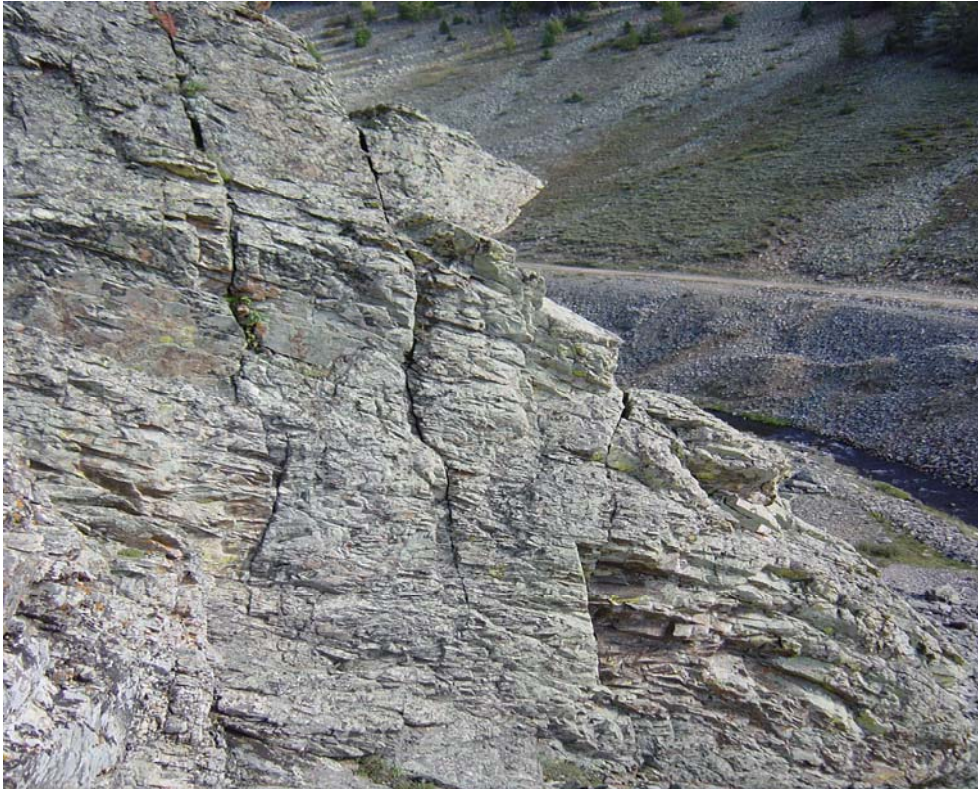
Photo 2.9 Joints of set J3 dipping towards the valley and opening of joints of set J2 due to gravitational effects on steep cliffs.
