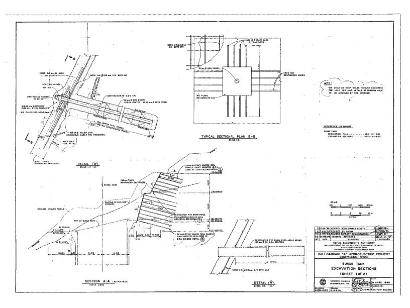
Surge Tank Cut Slope Rock Support Detail
