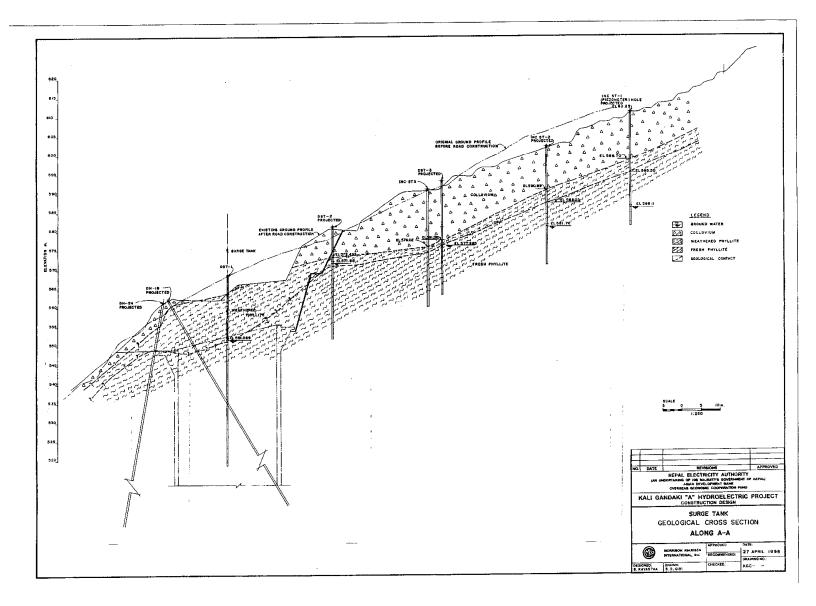
Geological X-Section of Surge Tank Cut & Back Slope
